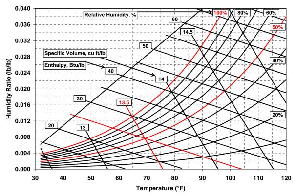
**Figure 22.** Psychrometric chart used to determine the physical properties air. Note that with values for only two parameters (e.g., dry bulb temperature and relative humidity, or dry and wet bulb temperatures), all others can be found in the chart (some interpolation may be necessary).
